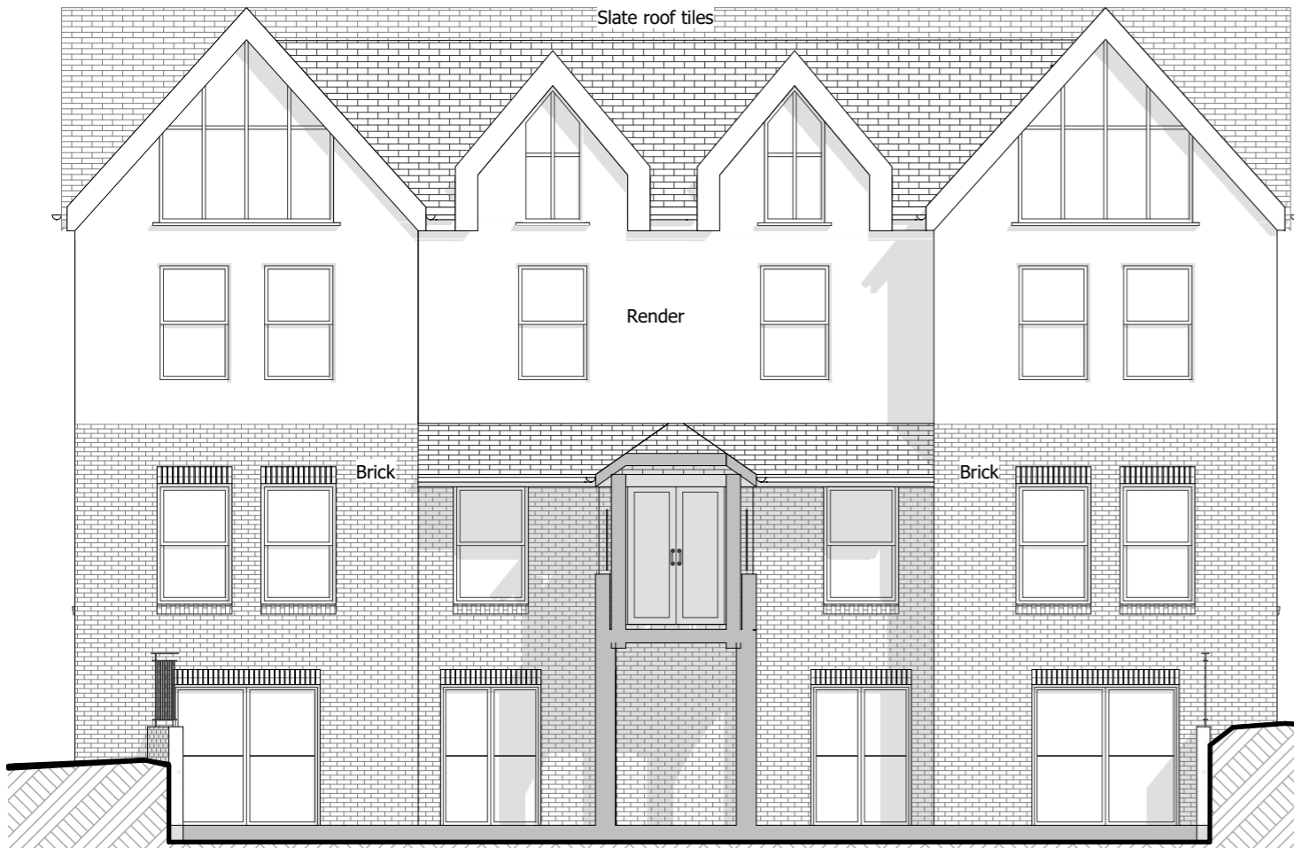
Front elevation/section from Lower Ground floor level
